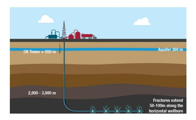
*Note*. This shows a well, drilling, and the process of hydraulic fracturing (or fracking). From the Canadian Association of Petroleum Producers, 2021 (<a href="https://www.capp.ca/explore/hydraulic-fracturing/">https://www.capp.ca/explore/hydraulic-fracturing/</a>).
