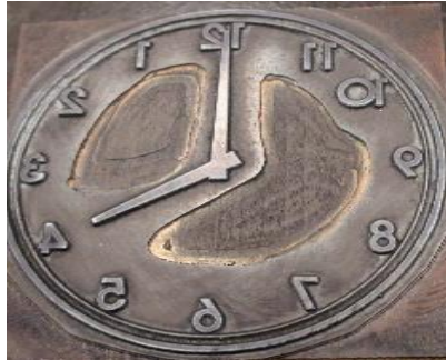
Figure 87. Print block of a clock with a reversed face. (2017). Image Credit: Amanda May.
